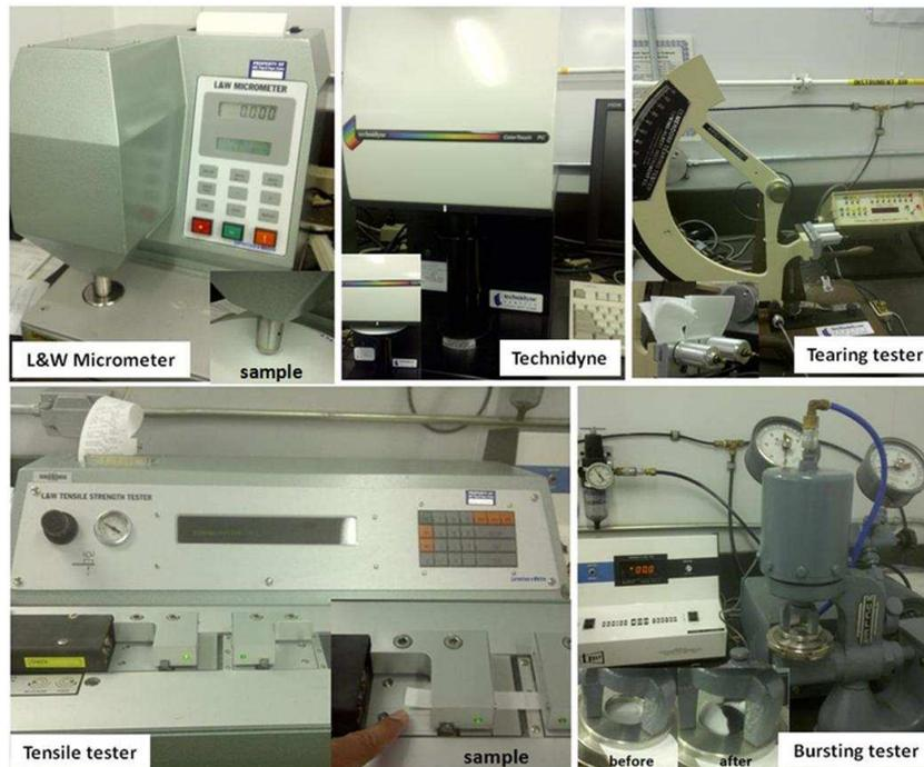
Figure 3.7. Apparatus for Measuring Paper Properties
