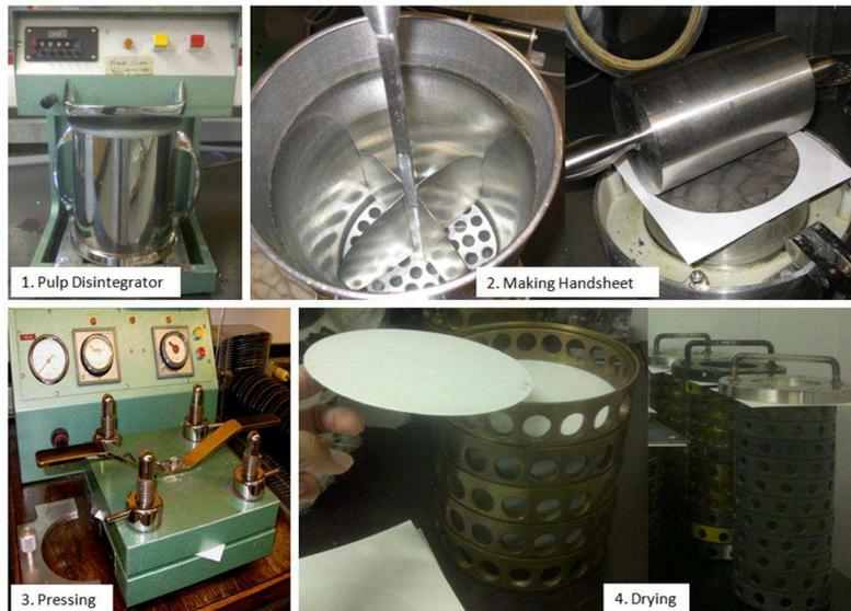
Figure 3.6. Handsheet Making Process: Steps for Making the Handsheet
